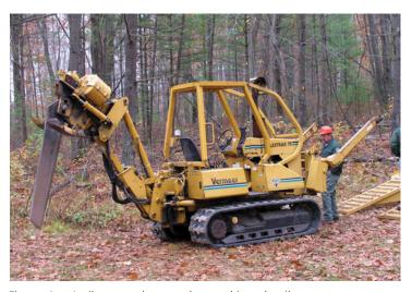
Figure 4.—A vibratory plow can be used in oak wilt management to disrupt root grafts and stop the fungus from spreading from infected trees to healthy trees. (U.S. Forest Service photo by Joseph O'Brien)
